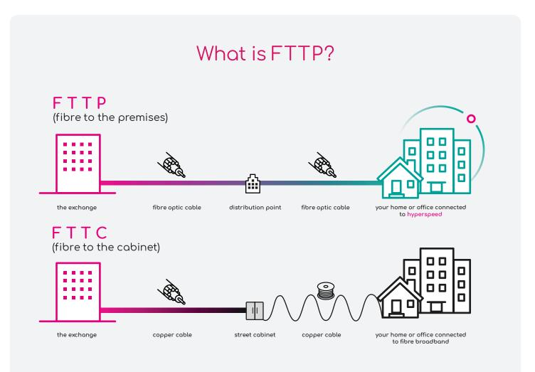
FTTP is a true end-to-end fibre solution – from the local exchange to the premises. Current UK footprint is 23.2% (as of June 21) and expanding month on month in line with the 2025 switch off campaign.
